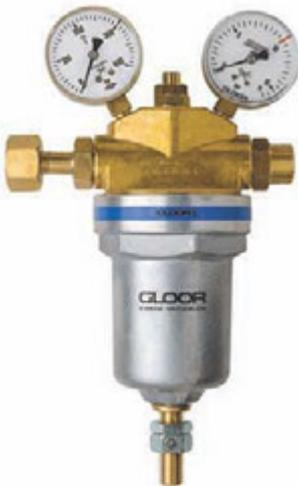
High flow rate pressure regulator (construction same as Art. 7900, but for inlet pressure up to 300 bar). With working pressure and contents gauges and integrated safety valve. Standard version with working pressure up to 10 bar. Also available with working pressure up to 20, resp. 30 bar (s.below).
