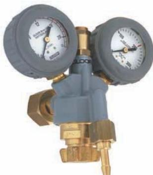
Mini pressure regulator with flow gauge, i.e. with indication l/min on secondary gauge. Integral safety valve. The flow is adjusted on the regulating screw by changing the secondary pressure and through a throttle valve in the outlet.
