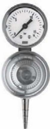
Pressure regulator with cylinder contents gauge. Flow rate with fully opened pressure adjusting screw alternatively 0.25, 0.5, 1.5 or 2.5 l/min. The pressure adjusting screw serves also as a shut-off valve. Particularly suitable for applications in which a precisely defined flow rate and secondary pressure are required.
