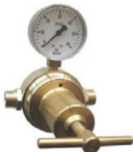
Low pressure regulator with mounted working pressure gauge and regulating screw for the adjustment of the working pressure up to 40 bar. Diaphragm made of NBR, filter in the inlet made of sinter bronze.
