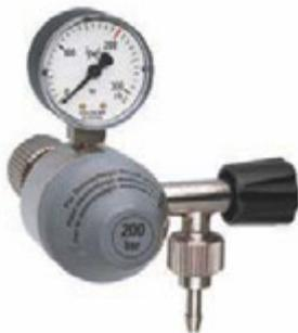
Pressure regulator with contents gauge for indication of cylinder pressure, but without working pressure gauge; with preset working pressure and integral safety valve. A fine regulation spindle enables a precise regulation of small quantities of gas (also for the aeration of aquariums).
