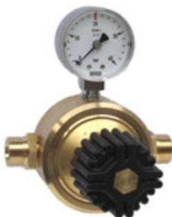
Low pressure regulator with mounted working pressure gauge and regulating screw for the adjustment of the working pressure. Diaphragm made of NBR, filter in the inlet made of sinter bronze.
